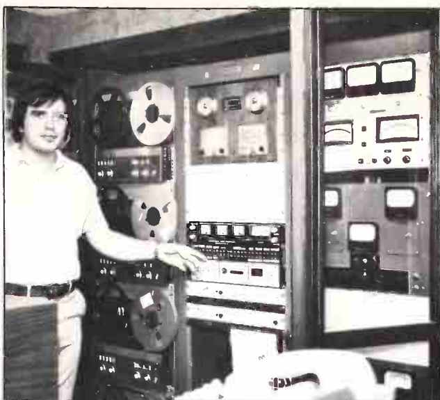
Tape decks, antenna monitor, EBS monitor, extended meter panel and other audio processing equipment in the main studio are behind two double-fold doors. Access also is available from behind and outside of the studio.
